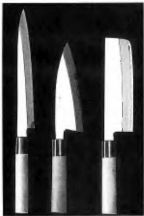
Three of the many specialized knives used by Japanese cooks: (l-r) yanagiba , deba-bocho , na-kiri bocho
